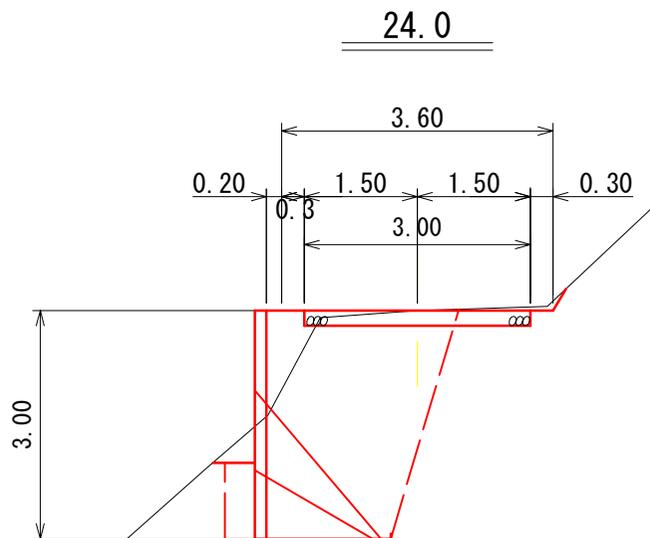
路盤工 =  $3.00 \times 0.10 \times 12.00 = 3.60\text{m}^3$
